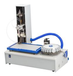
The width of the processed Sorbfil plates is up to 200 mm. The maximum amount of the applied sample is  $10~\mu l$ . The number of samples is up to 24. The application is performed by spraying the sample onto the Sorbfil plate with compressed air while the syringe is reciprocating along the direction of the sample application. The application of samples in the form of narrow lines ensures the highest achievable resolution in thin-layer chromatography.
