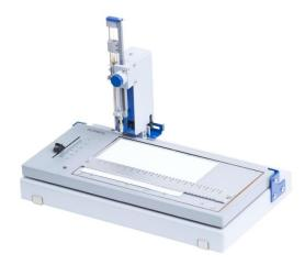
The sampler is used together with the USP-1 plates heater and the MSh-10 microsyringe with a guide that has a 40 mm long needle sharpened at a right angle.
